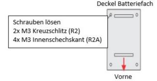
Illustration 1: Battery Case. Loosen screws. 2x phillips-tip screws (R2). 4x Hexagon socket (R2A). Front.
